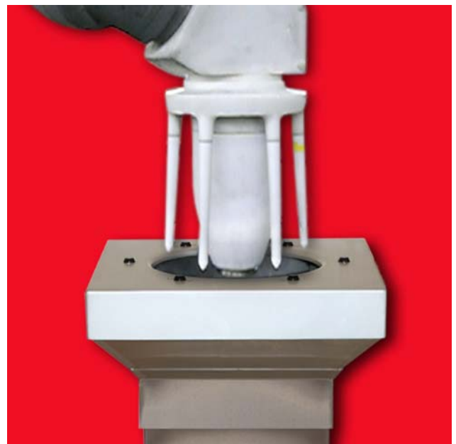
The Applicator Cleaner cleaning an externally charged applicator.
